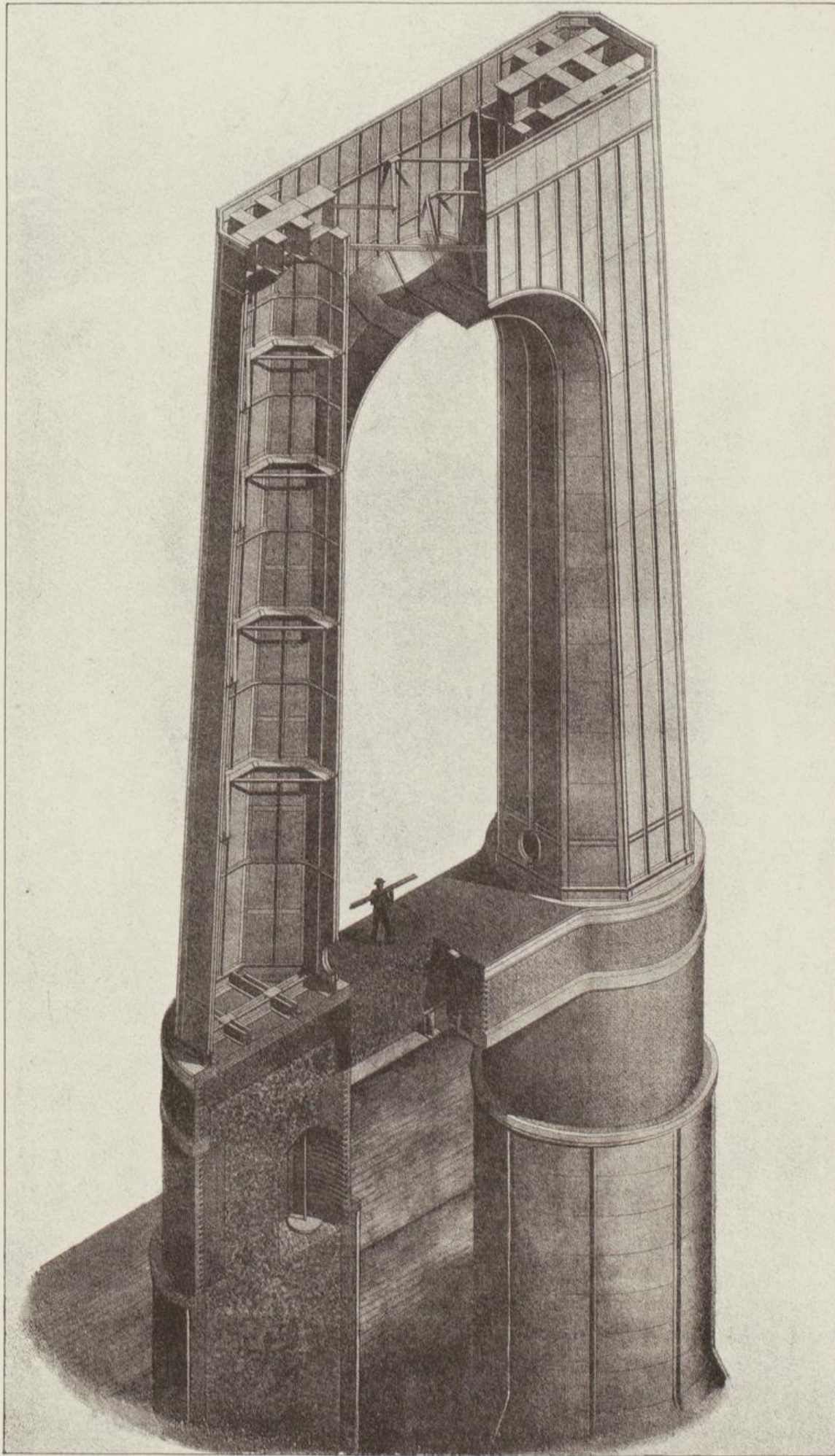
ISOMETRICAL DRAWING OF A PIER - TYPE II.
